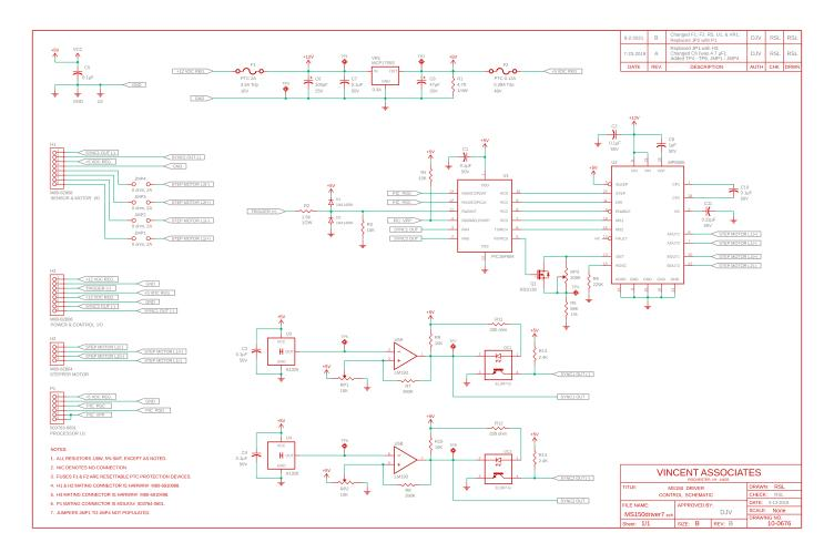
The above figure represents the schematic of the internal integrated driver. This shows the internal circuitry of the driver control board. The board is located under the actuator mount. This area also houses the open and close sensors. The sensors are Hall Effect type and determine the full-open and full-close status, while also doubling as the sync outputs that provide open and close signals.
