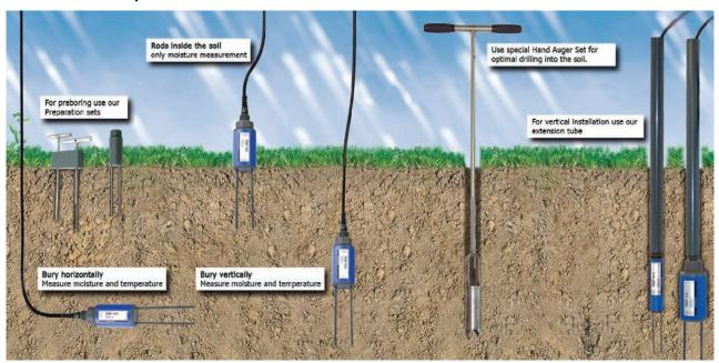
Conclusion: the probes should be permanently buried in the soil for optimum temperature measurement!
