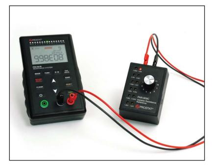
Using 1 percent tolerance resistors, the PAR-809C offers twelve values from  $1.2 \times 10^4$  to  $1.0 \times 10^9$ .
