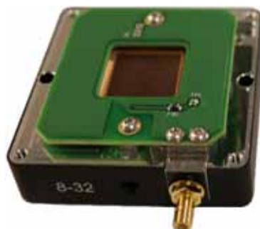
Figure 3-15. Align Pass-Thru Board in Sensor Housing
