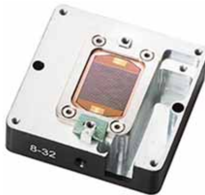
Figure 3-28. Retention Frame Secured
