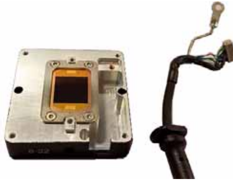
Figure 3-11. Remove Wiring Assembly from the Sensor
