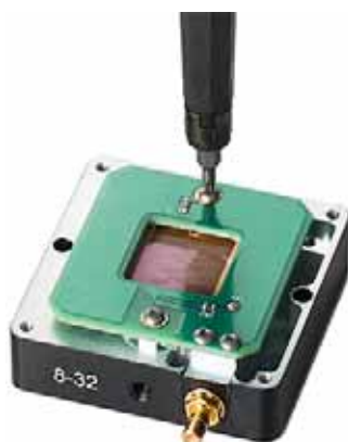
Figure 3-16. Attach Pass-Thru Circuit Board
