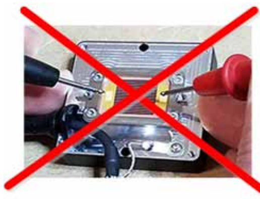
Figure 2-1. WARNING: Do NOT Probe the Sensor!
