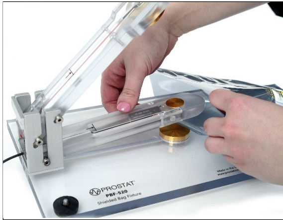
Figure 12. The Capacitive Arm inside the shielded bag.
