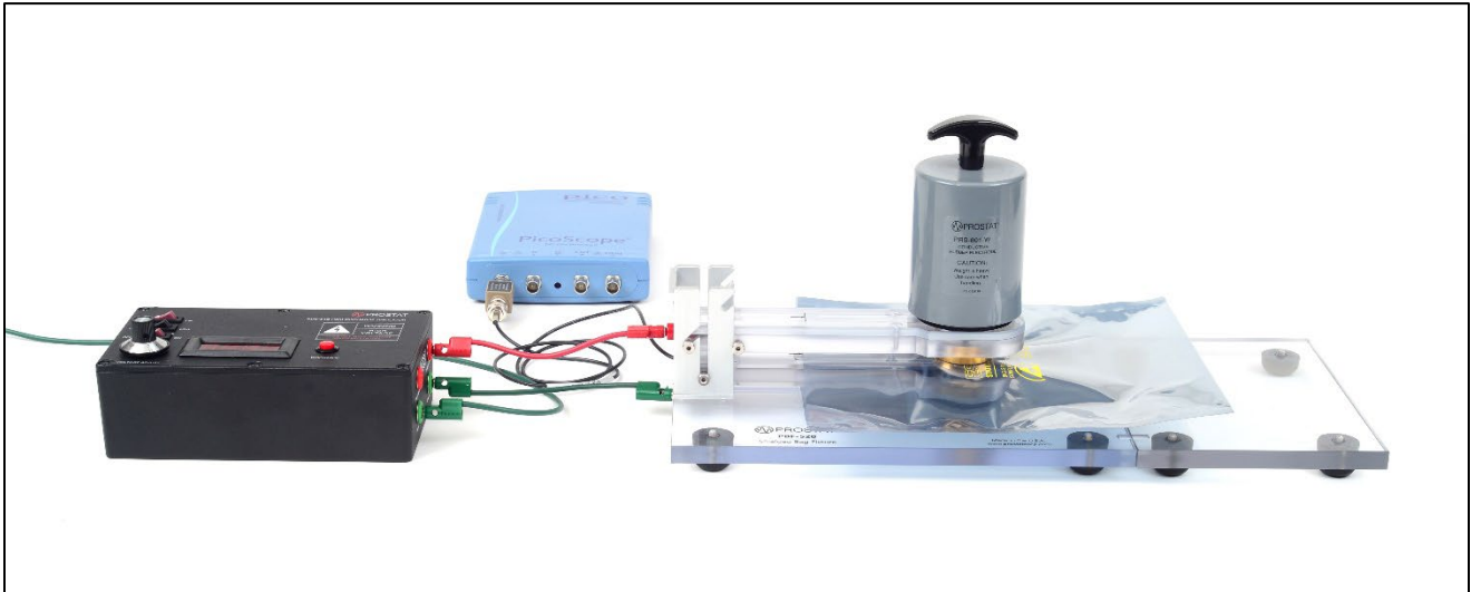
Figure 15. Complete setup for Shielded Bag Test.
