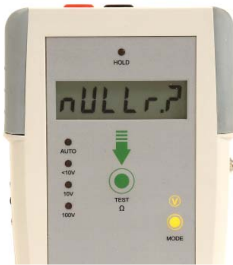
Figure 17: Press MODE to select NULL process
