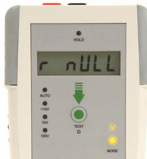
Figure 18: Press TEST and r nULL displays and starts
