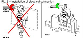
With the instrument into the final position provided that the electric line is not energize, remove the cover and make the electrical connection to the terminal block (see Fig. 2).
