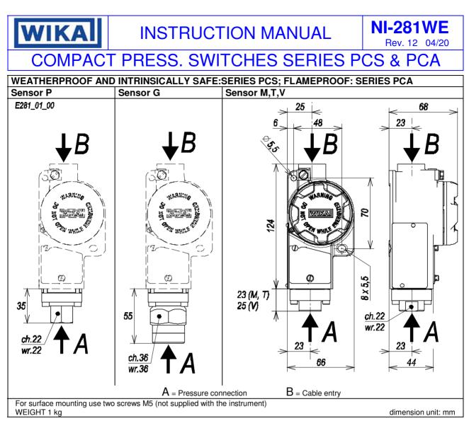
NOTE: dimensions and weights are not binding unless released on certified drawings.
