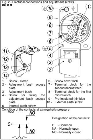
The effect of the direction of rotation of the adjustment bush is described on the adhesive label. Rotate the screw by inserting a 3.0 mm dia. rod into the holes of the adjustment screw (Fig.2).
