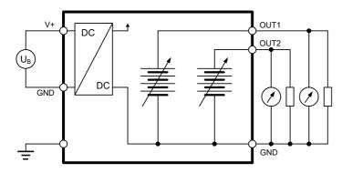
The maximum permissible cable length can be determined under consideration of the voltage drop caused by the current flowing to the devices connected to the unit. The voltage drop in the cable depends both on cable resistance and on the equivalent resistance of the devices connected in parallel to the unit. The total resistance connected to each unit output should be at least 1000  $\Omega$ . Cable resistance should not be more than 1/1000 of the load resistance.
