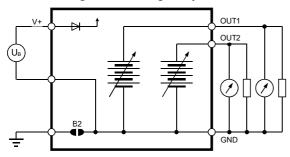
The maximum permissible cable length can be determined under consideration of the voltage drop caused by the current flowing to the devices connected to the unit. The voltage drop in the cable depends both on cable resistance and on the equivalent resistance of the devices connected in parallel to the unit. The total resistance connected to each unit output should be at least 1000  $\Omega$ . Cable resistance should not be more than 1/1000 of the load resistance.
