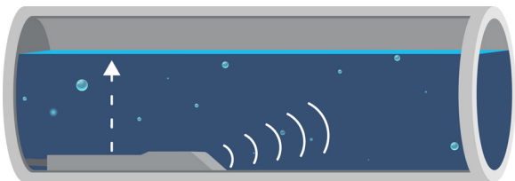
Submerged ultrasonic sensor measures level and velocity
