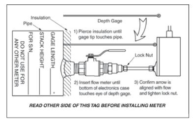
Prior to installing the meter, confirm that the stack height recorded on the tag is close to the actual stack height. Flow meter stems are intentionally oversized to allow for variations of at least 2" in the stack height. Contact GREYLINE prior to installation if there is any question regarding stack height or stem length. This way GREYLINE can offer you credit for your meter if you decide to exchange the meter for one with a different stem length. Returns may be subject to a restocking fee.
