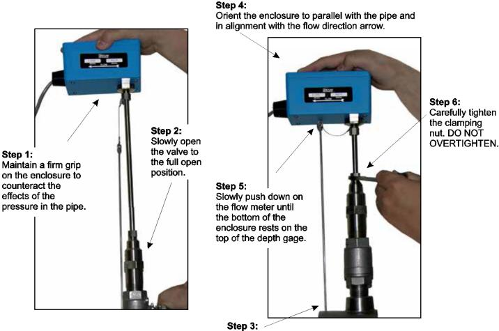
Use the end of the depth gage to pierce any insulation that may be present and rest the gage on the outside wall of the pipe.
