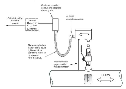
Install meter as shown using liquid-tight flex conduit and junction box. Leave sufficient slack in the liquid-tight flex conduit to allow the meter to be removed without disconnecting cable. Run factory installed meter cable to junction box above grade through liquid-tight flex conduit making connection to field wires at this point.
