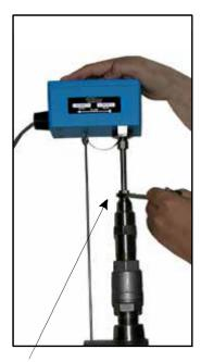
**Step 1:** Slowly loosen the position clamping nut while maintaining a firm grip on the enclosure to counteract the effect of pressure in the pipe.
