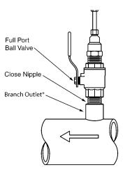
\*Weld-on fitting, copper tee or saddle
