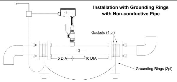
\* Additional straight run may be required upstream of the upstream grounding ring based on the nature of the upstream obstruction. Refer to the chart above to determine how much straight run is required.
