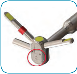
FlowTracker2 with optional integrated pressure (depth) sensor.
