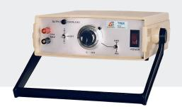
The Trek® 605A is a high voltage reference supply designed to provide precise control of output voltages in the range of 0 to +1 kVDC or 0 to -1 kVDC with an output current range of 0 to ±1 mADC. The Trek 605A provides two modes of operation: a fixed mode providing a constant +1 kV or -1 kV output, and a variable mode providing variable control of the output voltage with a one (1) volt resolution over a range of 0 to ±1 kV.
