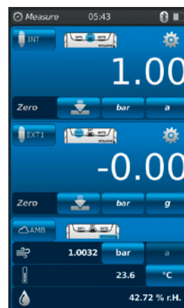
Representation of possible measuring channels
