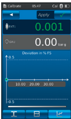
Representation of calibration results as graph
