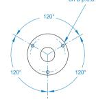
Pipe Mount 34 mm (1.34 in) diameter (standard 1 inch pipe) option with Terminal Strip Junction Box
