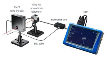
The RMC1 chopper should be mounted with the side marked "THIS SIDE TOWARD SENSOR" facing the RM9-PD. The side of the chopper blade facing this direction has a low emissivity surface. The other side of the blade faces the light source and has an absorptive black coating to minimize stray reflections.
