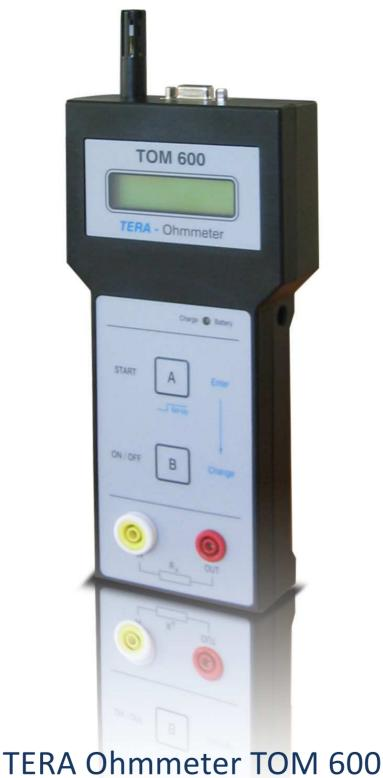
With integrated temperature and humidity sensor
