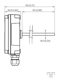
The TMI110 temperature transmitter is designed for measuring cooling/heating water temperatures in HVAC automation systems. When measuring the temperature of liquid, the transmitter is installed in a thermowell, as shown in this Quick Guide. For air temperature measurements, the transmitter can be installed in a duct using a flange.
