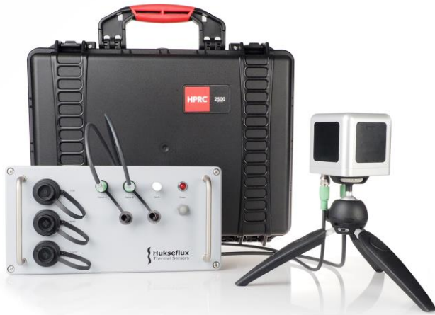
Figure 5 TCOMSYS01 with its TCOM01 sensor, tripod, MCU and carrying case
