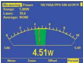
Analog needle display of power Persistence and min/max tracking.
