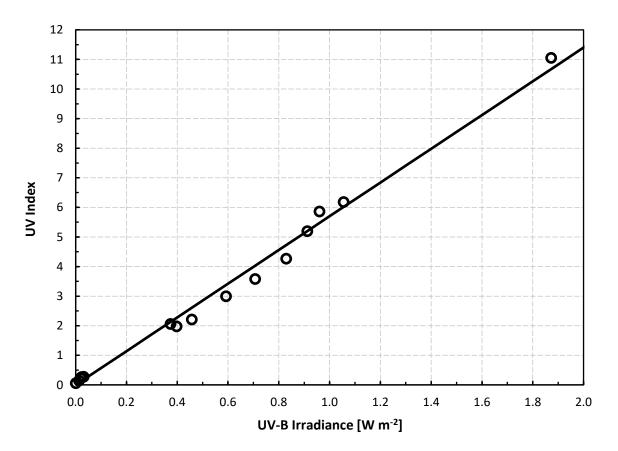
Relationship between UV Index and UV-B irradiance (in units of W  $m^{-2}$ ). Data are from multiple solar spectra representing a wide range of atmospheric conditions. Slope of the line is 5.7, with an  $r^2 = 0.99$ .
