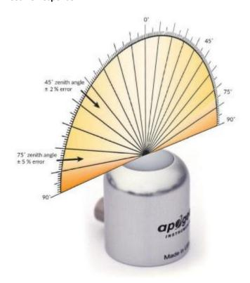
Directional, or cosine, response is defined as the measurement error at a specific angle of radiation incidence. Directional error for Apogee SU-300 series UV-I/UV-B sensors is approximately  $\pm$  2 % and  $\pm$  5 % at solar zenith angles of 45° and 75°, respectively.
