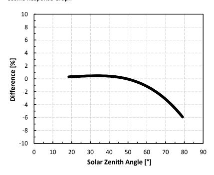
Mean cosine response of four Apogee UV-I/UV-B sensors. Cosine response was calculated as the relative difference of UV-I/UV-B sensors from a reference UV-I/UV-B sensor deployed outdoors. These data are the average of the AM and PM response.
