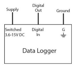
Figure 10: Pigtail End Wiring to Data Logger
