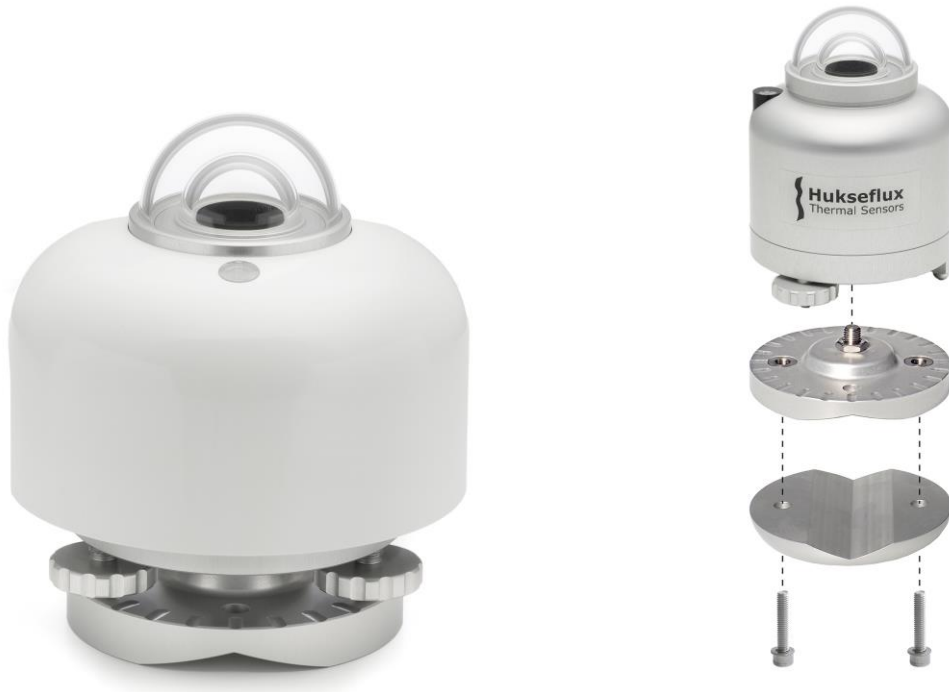
Figure 0.3 Optional levelling mount (picture on the left); a practical spring-loaded mount for easy mounting, levelling and instrument exchange on flat surfaces, and the optional tube mount (picture on the right) including spring-loaded levelling upper clamp, lower clamp for tube mounting and two sets of bolts
