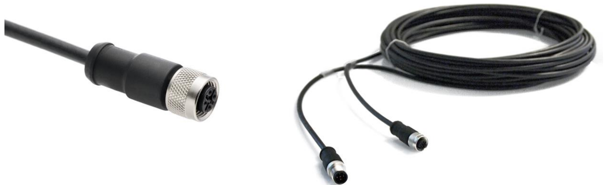
Figure 0.6 On the left the SR15 cable with M12-A female connector on sensor end, stripped over 0.15 m and conductors with ferrules. Its length is 5 metres standard and available in 10 and 20 metres too. On the right the optional Hukseflux extension cable with connector pairs, with male and female M12-A connectors, available in 20 metres
