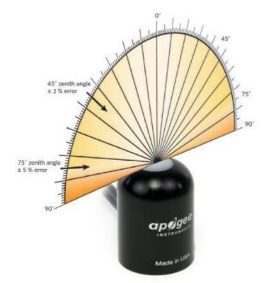
Directional, or cosine, response is defined as the measurement error at a specific angle of radiation incidence. Error for Apogee SQ-100X series quantum sensors is approximately  $\pm 2$  % and  $\pm 5$  % at solar zenith angles of 45° and 75°, respectively.
