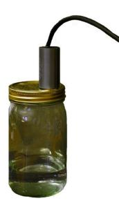
Apogee oxygen sensor mounted in a sealed chamber over water. For measurements in environments where relative humidity is 100 %, sensors should be calibrated in conditions where relative humidity is 100 % in order to account for any humidity effects on sensor electronics.
