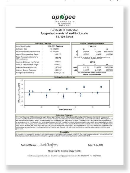
Calibration overview data are listed in box in upper left-hand corner, temperature errors are shown in graph, and calibration date is listed below descriptions of calibration procedure and traceability.
