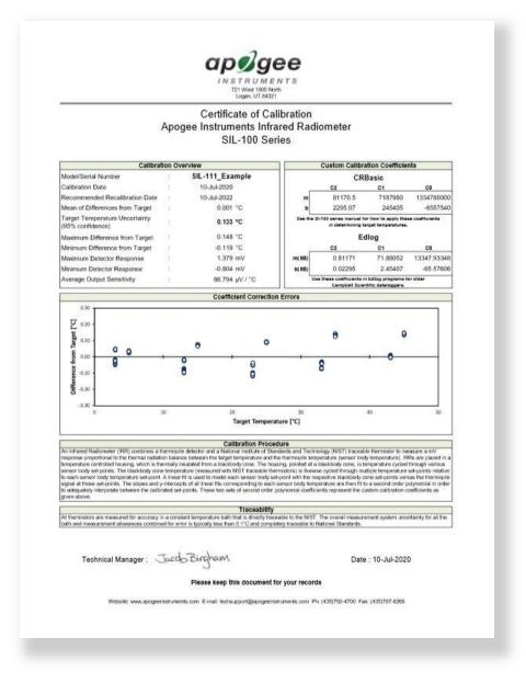
Calibration overview data are listed in box in upper, left-hand corner; sensor specific calibration coefficients are listed in box in upper, right-hand corner; temperature errors are shown in graph; and calibration date is listed below descriptions of calibration procedure and traceability.
