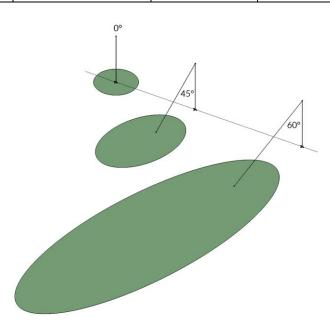
A simple FOV calculator for determining target dimensions based on infrared radiometer model, mounting height, and mounting angle, is available on the Apogee website: <u>https://www.apogeeinstruments.com/irr-calculators</u>.
