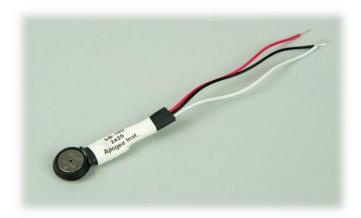
A sensor's model number, serial number, and production date are located on a label between the sensor and pigtail lead wires.
