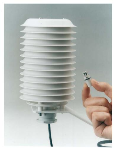
The RH and air temperature sensing elements are contained in a plug-in module. The module is interchangeable and can be replaced at routine maintenance intervals.
