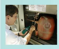
Compact meter is well-suited for field applications. Unique sensor cap closes for protection during storage. Simultaneously displays relative humidity, air temperature and dew point or wet bulb. Calculates T1-T2 differential (air temperature minus external probe temperature) using optional probe (TP890), and T2 minus dew point. Other features include Data Hold, Auto Power Off, and MAX/MIN reading.
