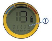
2 On the handheld device, select ▲ or ▼ to select the number of the receiver to pair.
