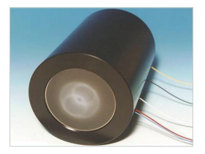
Demagnifiers are electrostatic focusing devices used for the detection of light particles where reduction in image size is required. The Photek Demagnifiers are available with either a 47 mm, 80 mm, or 150 mm diameter input window. They have high dynamic range, high resolution and are an efficient alternative to fibre optic tapers.
