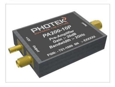
The PA200-10 preamplifier module is designed to be used with Photek detectors using 2 or less micro channel plates as they produce a small fast electrical pulse for each photon or particle passing through the detector.
