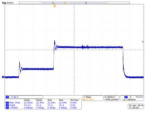
Internal trigger: 100 kHz, 2.5  $\mu s$  bias and 5.0  $\mu s$  main pulse width, 6 A bias current, 16 A main current.
