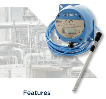
Intrinsically safe, surface mounted, two-wire loop powered oxygen analyser / transmitter with electrochemical sensor technology for 0-25% oxygen measurement.
