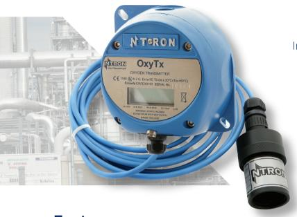
Intrinsically safe, surface mounted, two-wire loop powered oxygen analyser / transmitter with electrochemical sensor technology for 0-25% oxygen measurement.
