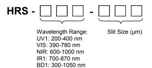
For example, HRS-VIS-010 is a spectrometer with a wavelength range of 390-780nm and a 10 μm slit size.
