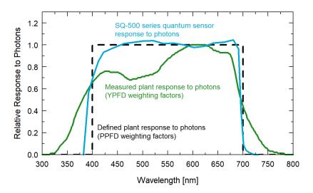
Defined plant response to photons (black line, weighting factors used to calculate PPFD), measured plant response to photons (green line, weighting factors used to calculate YPFD), and SQ-500 series quantum sensor response to photons (sensor spectral response).
