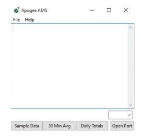
To establish communication, make sure the meter is plugged into your computer using the AC-100 communication cable. To connect click the dropdown menu button and "COM#" options will appear. For more details on how to figure out which COM is the right one,
