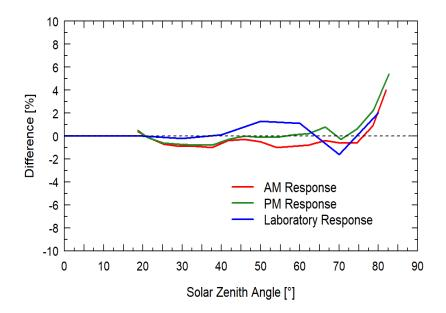
Mean directional (cosine) response of seven apogee MQ-500 series quantum sensors. Directional response measurements were made on the rooftop of the Apogee building in Logan, Utah. Directional response was calculated as the relative difference of MQ-500 quantum sensors from the mean of replicate reference quantum sensors (LI-COR models LI-190 and LI-190R, Kipp & Zonen model PQS 1). Data were also collected in the laboratory using a reference lamp and positioning the sensor at varying angles.
