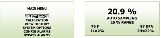
The display win some to the next higher range when the oxygen reading (actually the sensor's signal output) exceeds 99.9% of the upper limit of the current range. The display will shift to the next lower range when the oxygen reading drops to 85% of the upper limit of the next lower range.
