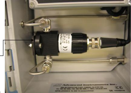
Delrin Housing with Oxygen Sensor installed
