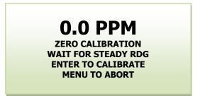
Pressing ENTER, the analyzer will complete ZERO calibration and return to Sample mode. If you press ENTER when the oxygen reading is outside of the acceptable zero offset limit, the analyzer will fail ZERO calibration and return to the Sample mode.
