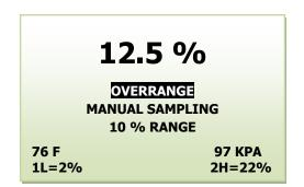
Once the OVER RANGE warning appears the user must advance the transmitter to the next higher range via the menu and keypad Press MENU, select MANUAL SAMPLING, press ENTER, select the appropriate MANUAL RANGE and press ENTER again.
