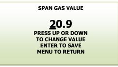
Press the ENTER key to advance the underline cursor right or press the MENU key to advance the underline cursor left.
