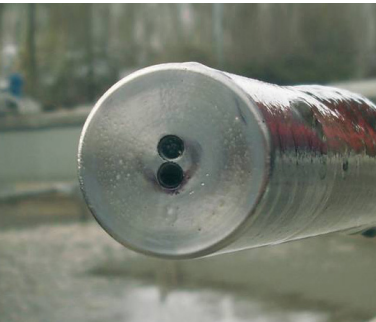
ViSolid sensor with UltraClean™ technology remains clean after a 30-day deployment.
