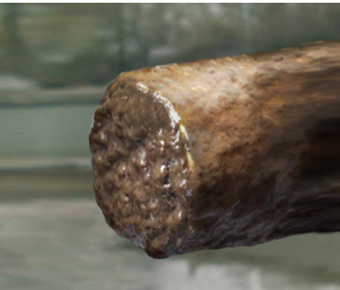
Dirty ViSolid sensor without UltraClean™ technology after a 30-day deployment.
