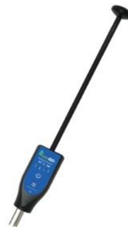
Figure 1.1. The portable HydraGO-FLEX and HydraGO-S allow for wireless on the go measurements of soil moisture. Connect via Bluetooth with a smartphone and the HydraGO App.
