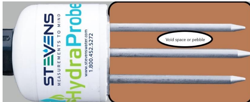
Figure 3.1 Measurement volume with a void space between the tine assembly.
