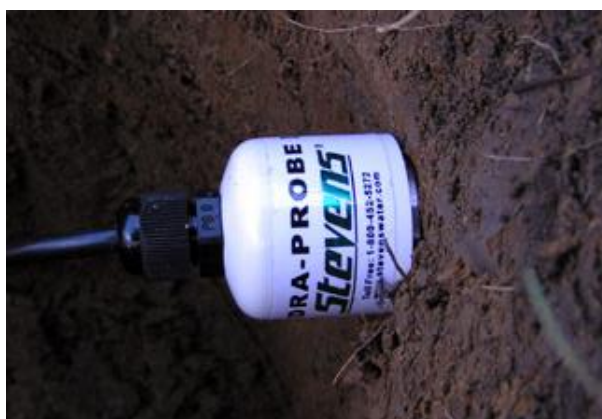
Figure 2.6 HydraProbe Installed in undisturbed soil.
