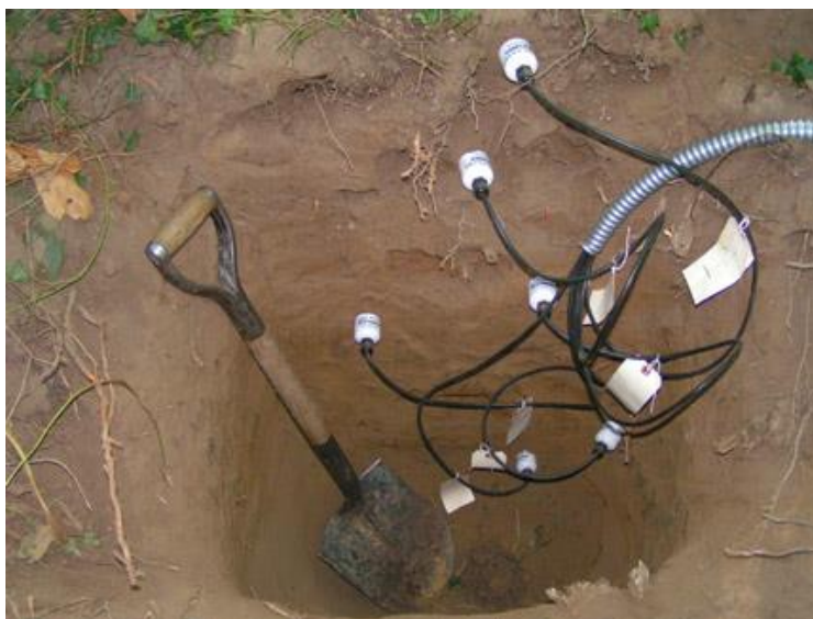
Figure 2.3 Six HydraProbes installed into 6 distinct soil horizons.
