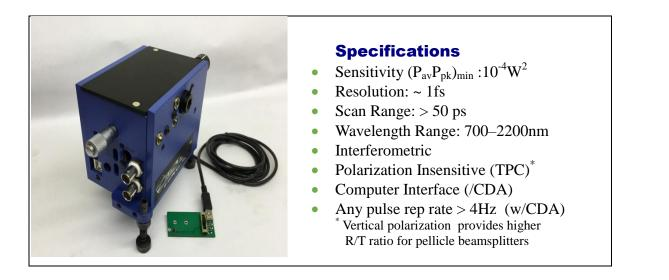
The **FR-103TPM** is a compact autocorrelator for Two Photon Microscopy applications. It can be introduced into the beampath of the laser without affecting optical alignment. The NL photosensor of the FR-103TPM can be placed in any location of the optical set-up, in particular at the position of the sample. Its Computer Data Acquisition (/CDA) option provides an interface (USB), for the display and analysis of autocorrelation traces on a Windows PC.
