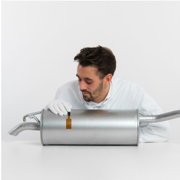
Figure 2 FHF06 high temperature foil heat flux sensor installed for measurement on a car exhaust pipe. The sensor is mounted on a curved surface.
