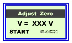
In this case adjust by the Zero Potentiometer on the back the Voltage to V < 0,10V
