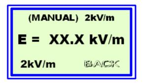
In the 1st. line it shows the selected Measure Mode  $\Rightarrow$  MANUAL and the Selected Range  $\Rightarrow$  2kV/m.
