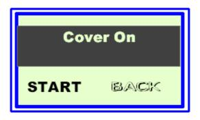
In the dark field it shows an advice to set the cover (protection cap) onto the modulator system. Press the "←→" Button (4) to select **START** or **BACK**.
