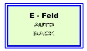
First the upper line is black. By pressing the "←→" Button(4) you can change the Mode. Selection => **E-Feld** => **V-Meter MK1** => **HV-Met.MK40** => **E-Feld** => etc.
