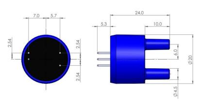
NOTE: 4.5mm OD push-fit tubing connectors.
