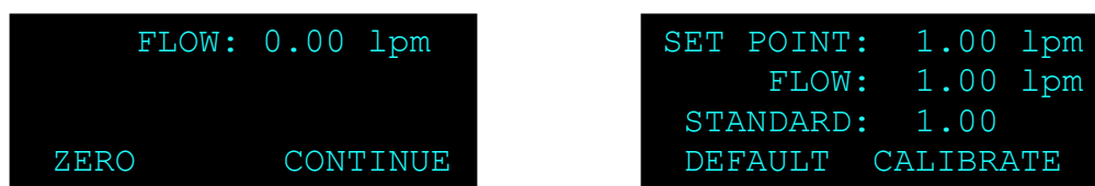
Figure 7-2 The C-12 Flow Calibration Screens
