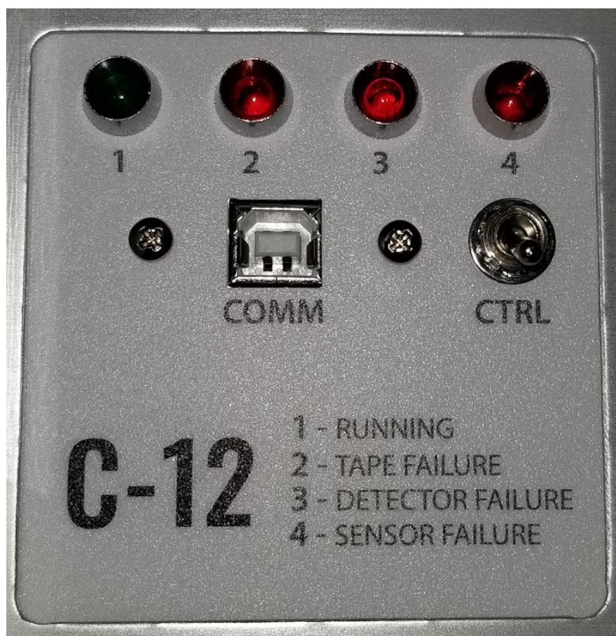
Figure 3-4 LED and Toggle Switch Interface
