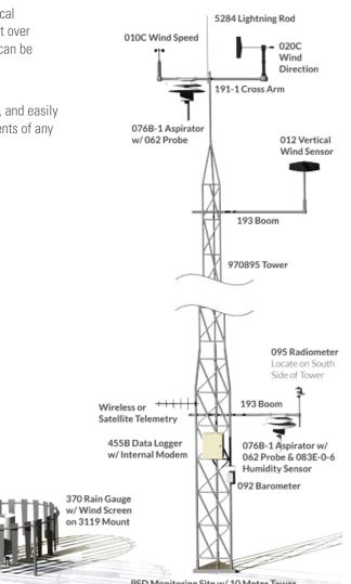
PSD Monitoring Site w/ 10 Meter Tower
