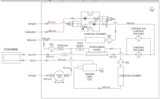
Figure 32 Pneumatic diagram with internal pump
