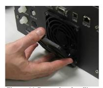
Figure 23 Removing fan filter
