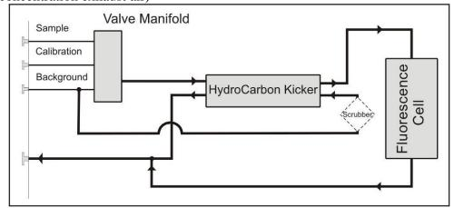
Figure 1 Simple pneumatic diagram
