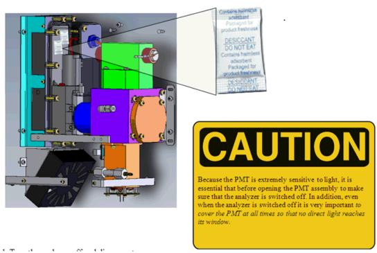
Figure 26 Position of desiccant packs
