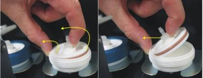
Figure 22 Removing plunger
