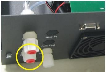
Figure 24 Plugged sample and calibration ports
