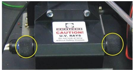
Figure 27 Collets of the UV lamp
