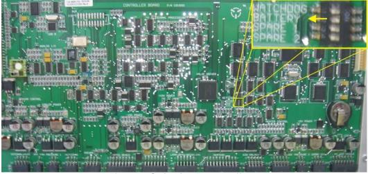
Figure 6. Switching battery off
