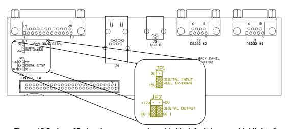
Figure 15 Serinus 25 pin microprocessor board (with default jumpers highlighted)
