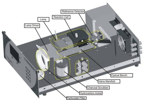
Figure 3 Major Components of analyzer
