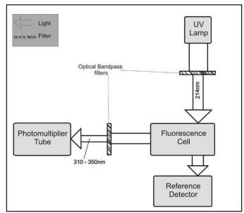
Figure 2 Optical measurement theory
