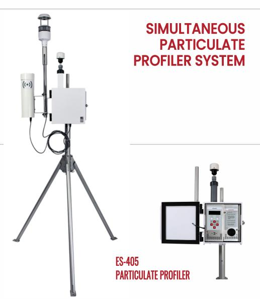
Met One Instruments, Inc. AQ EAGLE is a system utilizing our ES-405 Particulate Profiler. The ES-405 continuously samples ambient air and reports particulate mass concentrations simultaneously and in real time for PM<sub>10</sub>, PM<sub>4</sub>, PM<sub>2.5</sub> and PM<sub>1</sub>. Our ES-405 is ideal for fugitive emissions and neighborhood scale community monitoring projects where both simple operation, portability and modest cost of
