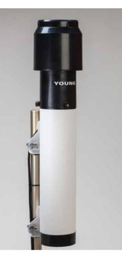
When the column level reaches a maximum of 250 mm (50 mm of precipitation), the chamber automatically empties and the process repeats. Total precipitation can be tracked by a datalogger or recorder.
