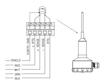
**NOTE:** The terminal marked "EARTH GND" should be connected to properly grounded tower, or grounding conductor, as close to the sensor as possible. Failure to do so may result in damage due to static discharge.
